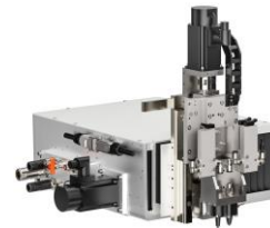
The 315 marking unit with motorised Z-axis
